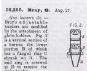
1894. The Bray patent burner.
