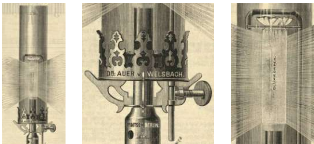
1886. Made by Julius Pintsch, Berlin. The first gas mantle burner of Dr. Auer von Welsbach.
